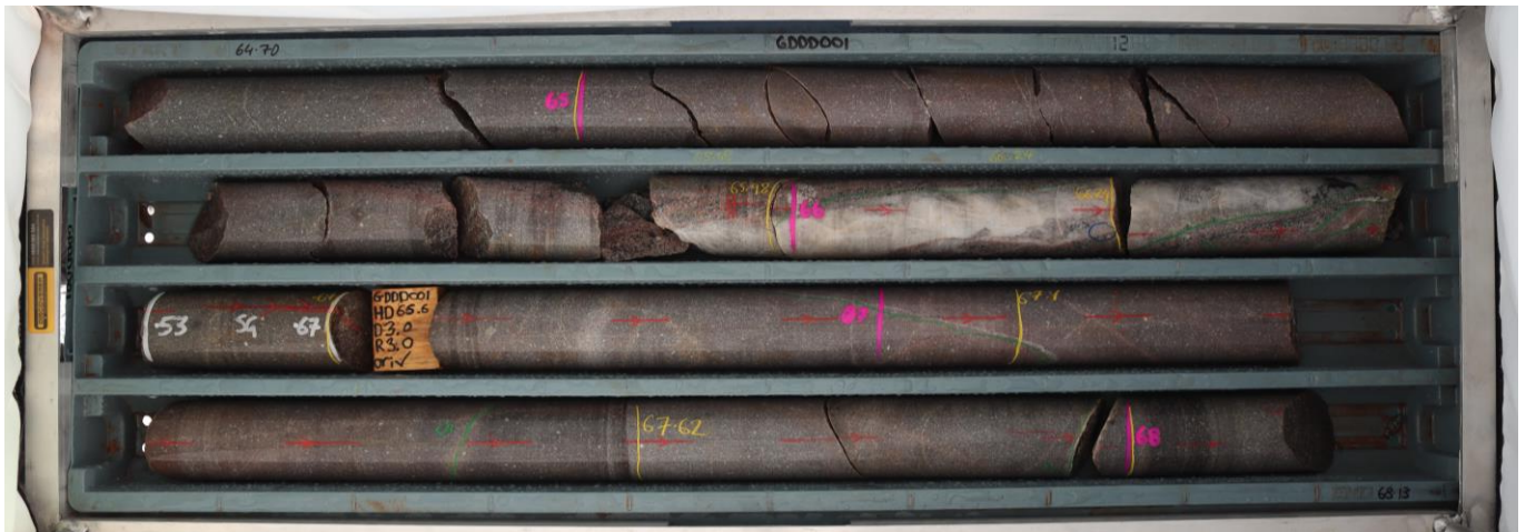
Figure 4. GDDD001 (64.7m – 68.13m) showing low-angle quartz vein containing coarse visible gold, within a felsic porphyry.
