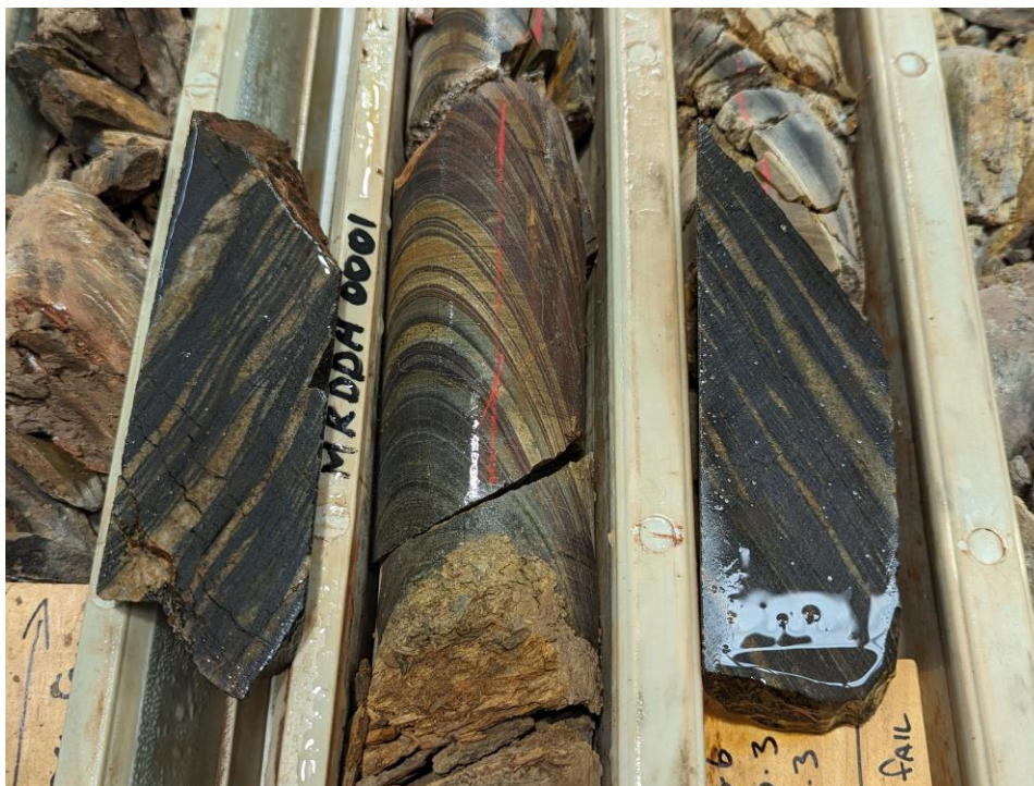
Figure 6. Comparison of magnetite-rich banded iron formation from the Cleaverville Formation (centre) with samples from historic Whaleshark diamond drill holes (left and right).
