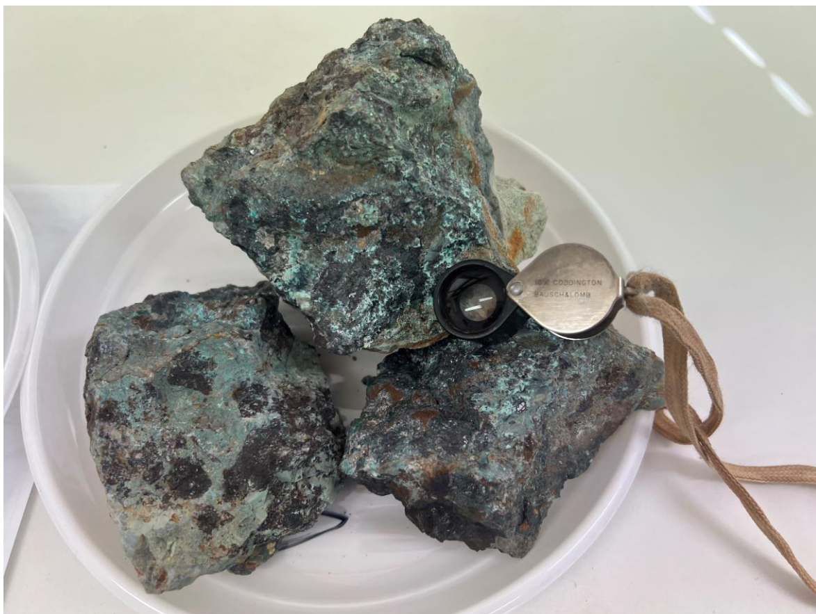
Figure 1. Sample CP003 (5.49% Cu, 42%Pb, 73.48g/t Ag) showing malachite (green), galena (shiny grey) and sphalerite (grey-brown).
